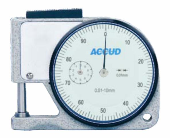
◆ Stainless steel spindle tip and anvil
