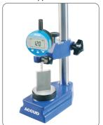
Rigid construction, designed to make comparison height measurement (set zero with gage block then measure height of workpiece) with dial indicators or digital indicators (variation of measuring force is high)
